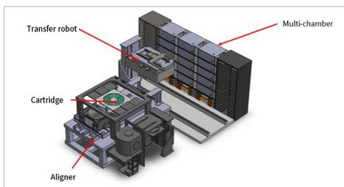
Picture 1 High-speed multi-probing wafer inspection system schematic diagram and cartridge
