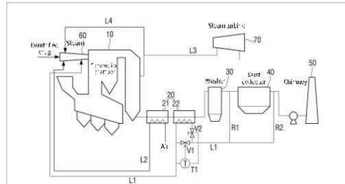
Figure 2 Nitrogen oxide removal system
