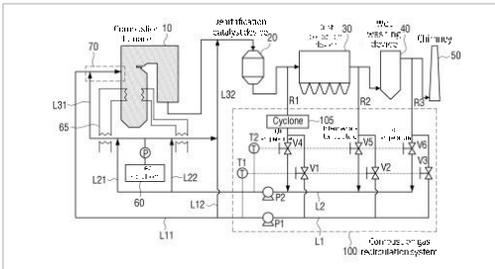
Figure 1 Combustion gas processing system using multi-stage combustion gas recirculation
